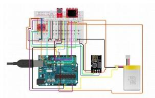
For sending automated messages to authority, GSM module was integrated with Noise measurement system above.
