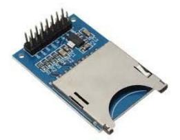
The SD library allows for reading from and writing to SD cards, e.g. on the Arduino Ethernet Shield. The communication between the microcontroller and the SD card uses SPI, which takes place on digital pins 11, 12, and 13 (on most Arduino boards) or 50, 51, and 52
