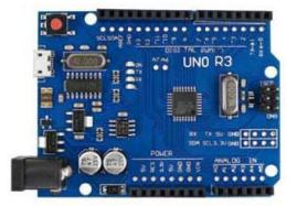
The Arduino Uno is an open-source microcontroller board based on the Microchip ATmega328P microcontroller and developed by Arduino.cc. The board is equipped with sets of digital and analog input/output pins that may be interfaced to various expansion boards and other circuits.
