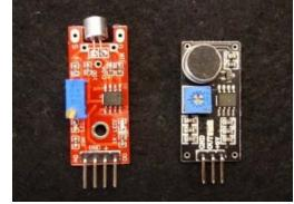
Microphone sound sensor: It gives a measurement of how loud a sound is.
